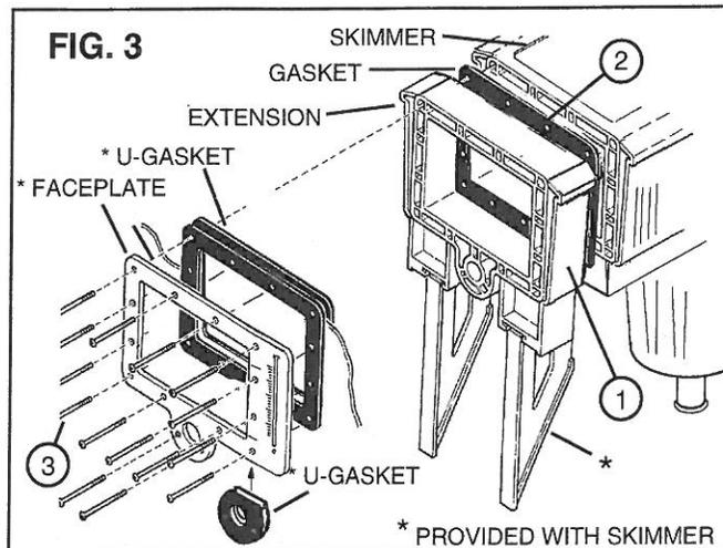
6. Insure that both inside and outside gaskets are aligned and in contact with the flanges of the faceplate, extension, and skimmer. Using the faceplate as a guide, pierce the remaining 13 screw holes in the liner. Insert the remaining screws just enough that the screw threads begin to thread into the skimmer/skim filter body. Firmly tighten all screws evenly, alternating left to right and top to bottom, until all screws are tight.
