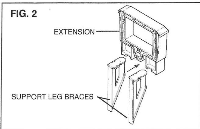
2. The skimmer extension has two alignment tabs that will slide into the slots under the faceplate of the skimmer/skim filter. Align a gasket with the extension over the tabs. Slide the tabs of the extension into the skimmer/skim filter so that the gasket aligns between them. Set this assembly aside for now.
