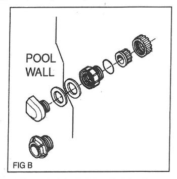
2. Slip a gasket over the threads of the return fitting (included with skimmer) and push threaded end through the wall from the inside. Place a second gasket over the threads exposed outside of pool wall. Thread UNION ADAPTER (Item #5), onto return fitting and
