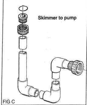
4. Route and plumb PVC pipe for Return to Filter and pre-assemble prior to gluing and check for fit. Place Union nut (Item #3), over pvc pipe prior to gluing Union socket (Item #2). See FIG D for typical plumbing installation.
