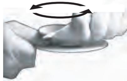
3) Twist the Step Cup™ to ensure that its mushroom has entirely cleared the wall thickness. If it has, the suction cup should rotate freely.
